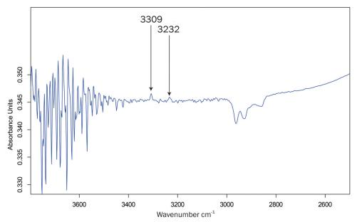
**Fig. 3** Infrared spectrum of the same Madagascar pink sapphire using the DRIFTS (diffuse reflectance) attachment. This bounces the beam through the gem from a variety of directions. Using this technique, the 3309 cm<sup>-1</sup> rises well above the noise floor. In addition, the peak at 3232 cm<sup>-1</sup> rises above the noise floor, proving that the gem had been subjected to artificial heat treatment.
