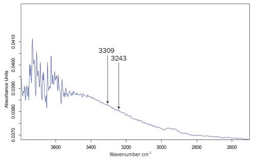
**Fig. 2** Infrared spectrum of a Madagascar pink sapphire using the Pike 4x beam condenser collection attachment. This sends a narrow beam through the gem. Using this technique, the 3309 cm<sup>-1</sup> was at the noise floor, while the 3232 cm<sup>-1</sup> peak was not visible at all.
