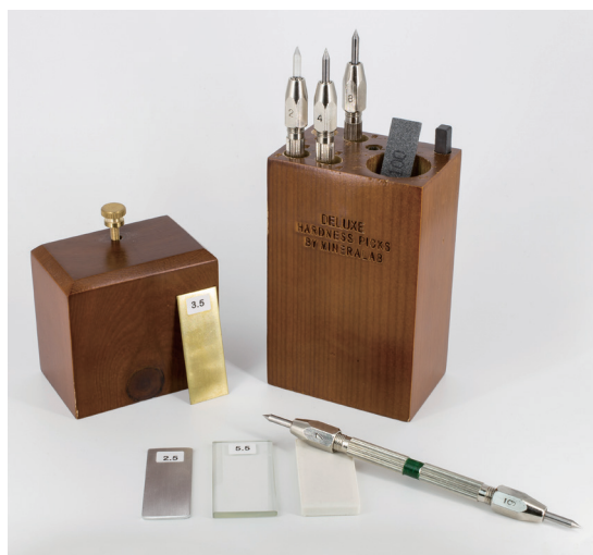
Fig. 10 A Mohs hardness scratch testing kit.
