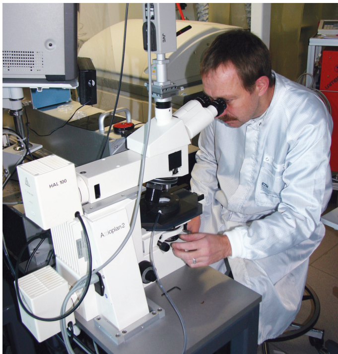
Figure 4. Author Detlef Günther analyzing fluid inclusions with a 193 nm ArF excimer ablation system coupled to an ICP-MS for the elemental analyses.
