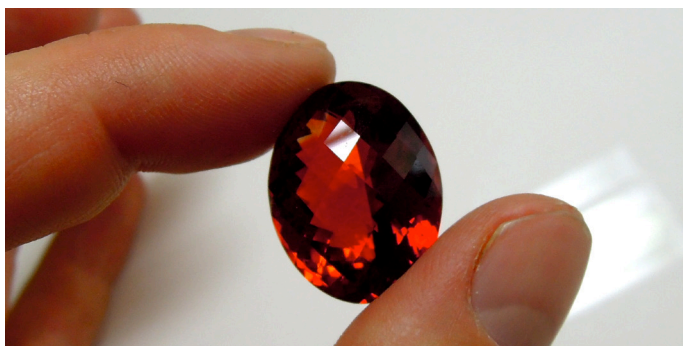
Figure 9. Copper-bearing andesine such as this 25.86-ct stone is sold around the world as Tibetan. It is likely that most of this material is diffusion treated.
