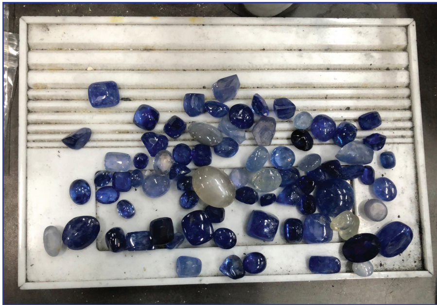
Figure 2: This parcel of sapphires (mostly heated) before treatment reveals the wide color range of the starting material. (Photo: Shane McClure, GIA)
